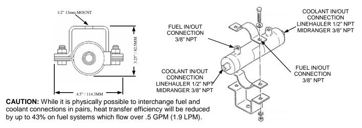
**MOUNTING:** Using appropriate mounting hardware, the in-line fuel warmer can be frame or engine/transmission mounted in either the horizontal or vertical position. To provide maximum cold weather protection, the in-line warmer must be I; located as close as possible to the primary fuel filter. Some engine applications may not be equipped with a primary fuel filter between the tank and transfer pump. In this situation, locate warmer as close as possible to the transfer pump.
